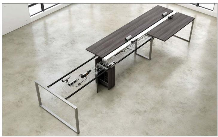
Steel beams running between the support legs give lateral strength to the bench while supporting the worksurfaces. Steel or laminate intermediate legs can be used to provide support for longer runs. The 8-wire, 4-circuit electrical can be placed in the wire basket under the worksurfaces.
